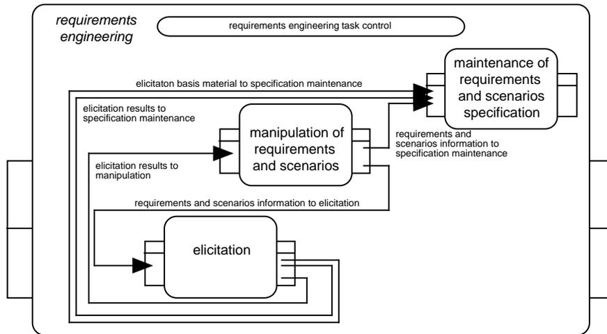
**Figure 2.** Process composition of requirements engineering: information links
